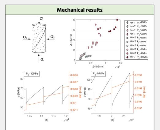
Stick-slip events were induced at different confining pressures ( $P_c$ ). A linear mutual dependence was observed between shear stress drop and associated slip.
