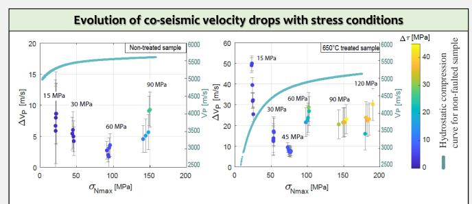
$\Delta V_P$  observed in the non-treated sample are visibly smaller than the ones observed in the treated sample (i.e. higher initial damage degree).
