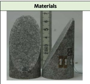
Damage zone elastic properties were simulated with thermal treatment (i.e. inducing intense microcracking), producing different degrees of damage in the samples' bulk.
