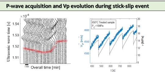
Elastic waves travelling across the sample were continuously recorded during the experiments. P-wave arrival was automatically detected and P-wave velocity estimated ( $V_p$ ). An increase in  $V_p$  was observed during hydrostatic increase of  $P_c$  and during differential loading. Drops in  $V_p$  ( $\Delta V_p$ ) occurred during stress drops.
