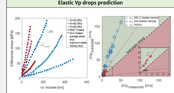
Elastic  $\Delta V_P$  were predicted by comparing differential stress increase with the total  $V_P$  increase during elastic loading right before instability occured. A linear dependence between  $\Delta V_{P \text{ predicted}}$  (i.e. drops due to the opening of the cracks present in the bulk of the sample, caused by the only stress release) and  $\Delta V_{P \text{ measured}}$  was observed.
