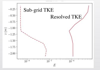
For example, the sub-grid scheme Dynamic Smagorinsky depletes TKE close to the ice base due to the combination of the boundary and strong stratification. The choice of sub-grid scheme is not obvious
