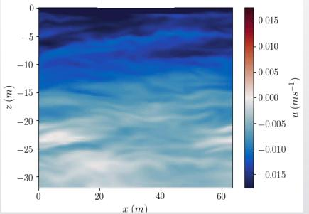
Simulation output with stabilizing stratification and ice-shelf melting and horizontal flow is primarily driven by background pressure gradients.
