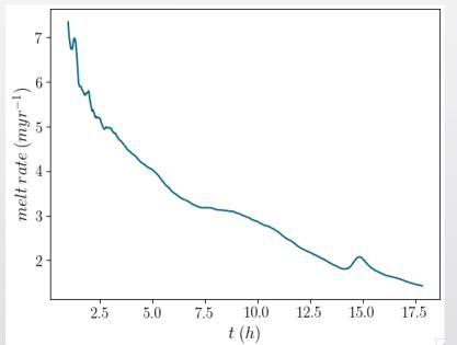
Melt rate timeseries from a simulation in which stratification increases through time resulting in steadily decreasing melt rates.
