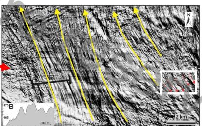
Yellow arrows indicate ice flow direction parallel to the longest axis of the Woodfjorden Trough.
