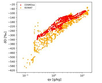
COSMOiso vs. ground-based remote sensing (FTIR) retrievals for 4.9 km (representative of 3-7 km)
