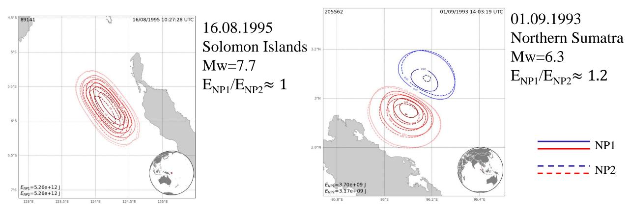
Calculations of forms of initial water elevation with use of NP1 and NP2 data sometimes provide very close results
