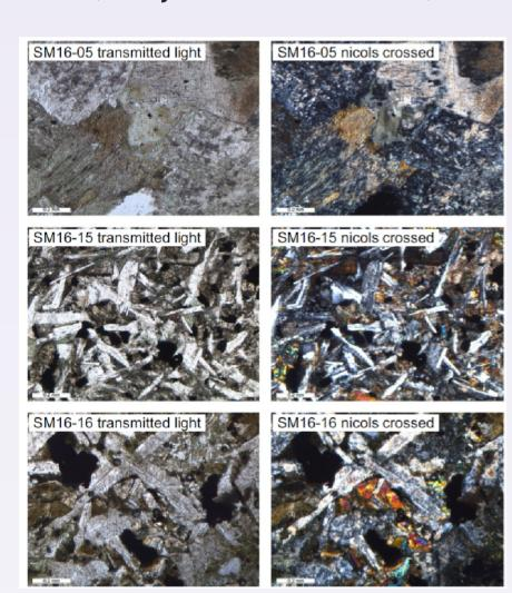
Transmitted (left) and polarized (right) light microscope images of thin sections of some of the studied samples
