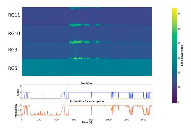
Similar to the example shown in the last slide here we show a classification example from our Turrialba data set. Class 0 is noise, class 1 is eruption, class 2 is rain. One can see clearly that the network has difficulties to determine the exact end of an eruption (usually dominated by ash falling back onto the ground) or even finds more eruptions than human-picked.
