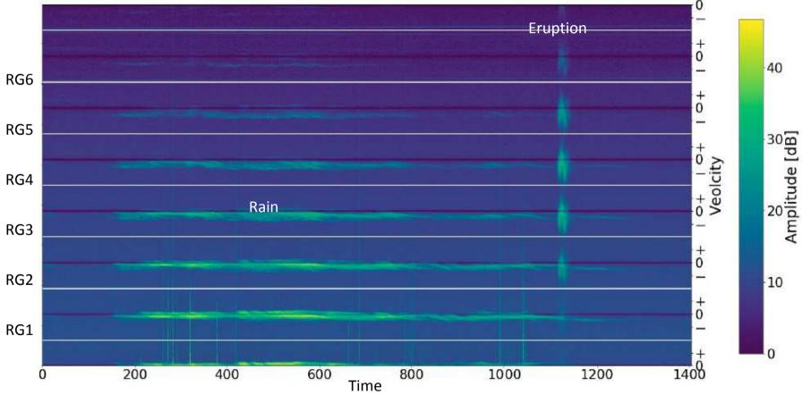
Recording of an eruption at Volcan de Colima volcano during rain. Shown is the full set of data recorded by the radar (Range Gates 1-6). They are separated by the white horizontal lines. Due to spectral leaking in the radar during data processing the eruption (occurred in Range Gate 5) is also visible in range gates 3, 4, and 6.
