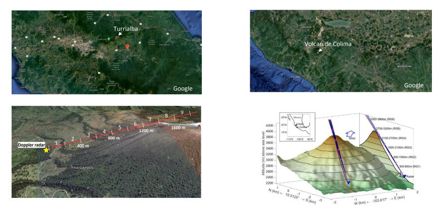
For recording the data we use a Frequency Modulated Continous Wave Radar. Range Gate resolution in case of Turrialba was 200 m and range gates RG5, RG9-RG11 were recorded . In case of Volcan de Colima we used a range gate length of 600 m and range gates RG1-RG6 were recorded. Data at Volcan de Colima were recorded in 2014/2015 and at Turrialba volcano data was recorded between July 2017 and Jan 2019.
