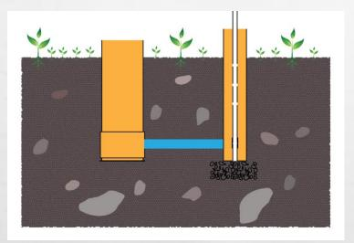
**Figure 3.** A single core (left) connected to the water table management pipe/reservoir on the right
