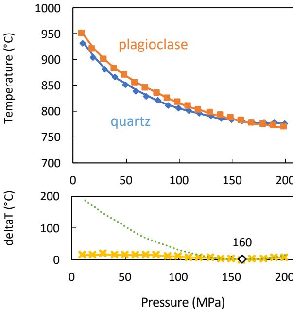
**Calculations for this sample reveal equilibration pressures of 126 - 160 MPa**
