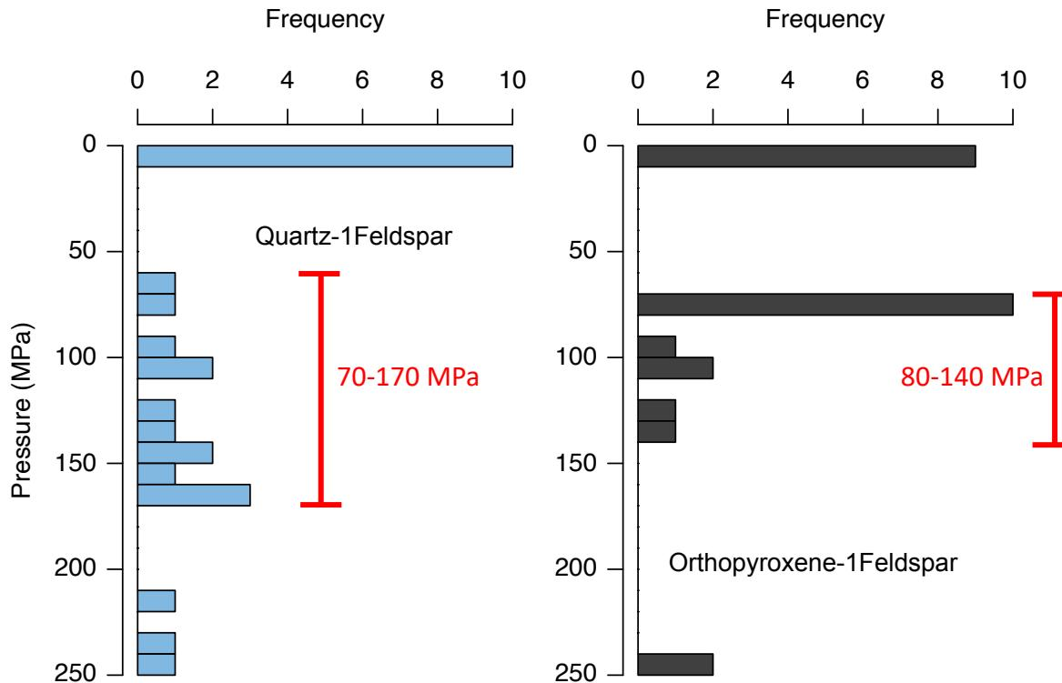
Equilibration pressures are calculated for all melt inclusions and pockets using two rhyolite-MELTS barometers (qtz-plag & opx-plag).
