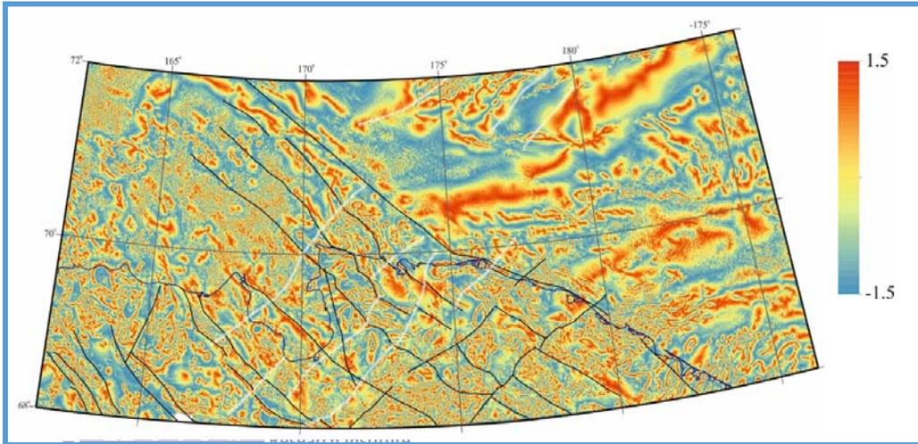
*For tectonic elements mapping we used high-pass filtered maps, horizontal derivative and tilt-derivative of potential field data. The known thrusts of NW direction (black lines in the maps) are detected clearly. In addition the NE oriented faults could be delineated (white lines).*
