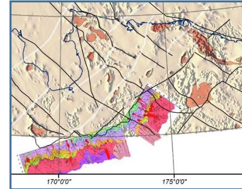
Segment of the horizontal derivative magnetic map and geological section along 2DV according to joint interpretation results. The NW oriented faults are sub-vertical but have a tendency to dip in the NE direction.
