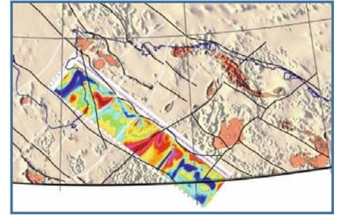
Segment of the horizontal derivative magnetic map and 2DV-A geoelectric section. The NE directed faults connected with sub-vertical conductive anomalies.
