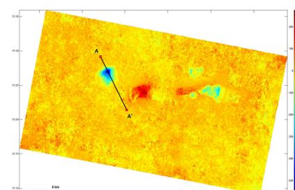
Fig. 12. Small Baseline InSAR cumulative map of subsidence of the mining area. The profile of subsidence A-A' is shown in Fig. 15 (a).
