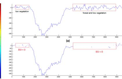
Fig. 15. The profile of subsidence A-A' presents the plot of cumulative land subsidence of the total analyzed period of time.
