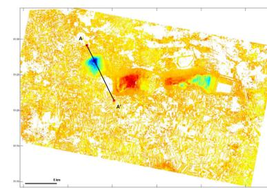
Fig. 14. BSI-SBAS cumulative map of subsidence of the mining area. The profile of subsidence A-A' is shown in Fig. 15 (b).
