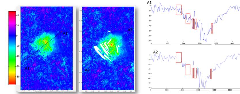
Fig. 17. An example of a spreader machine working on the dumping area C. The profile A1-A1' (left) the final SBAS results of cumulative ground subsidence and (right) image with profile A2-A2'.
