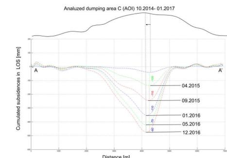
Fig. 16. The plot of cumulative LOS displacements on AOI dumping area C in analyzed period of time.
