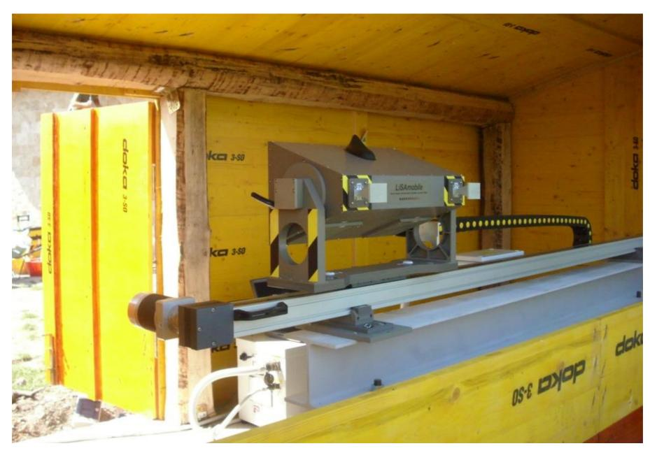
Modern GB-InSAR apparatuses, capable of acquiring in less than one minute, enable the early warning of rigid (brittle) rock failures
