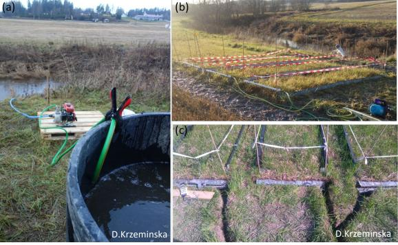
**<u>Runoff simulation setup</u>**: (a) water from the stream was pumped to a tank and mixed with slurry to a known suspended sediment concentration; (b) the mix was distributed upslope of the experimental plots by *line irrigation; (c) surface runoff was collected downslope* and laboratory analyzed for: suspended sediment, total phosphorus, total nitrogen, organic matter and *clay content*.
