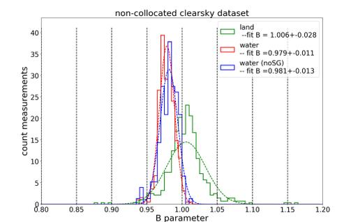
Figure 5: Fit results of dataset 2 for different surfaces using a fit parameter B and an additive offset C.
