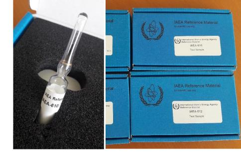
2. New carbonate RMs covering range of  $\delta^{13}$ C values, IAEA-610, IAEA-611, IAEA-612
