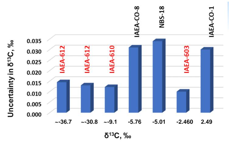
The combined uncertainty estimated for new RMs (these are marked in red) includes the uncertainty components related to the material homogeneity, stability, mass-spectrometer' linearity and cross-contamination.
