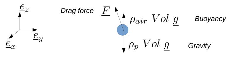
$$\underline{F} = \frac{1}{2} \frac{\pi D^2}{4} c_D \rho_{air} v_{rel} \underline{v}_{rel}$$
