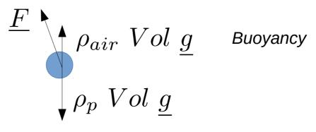
$$\frac{d\underline{v}_p}{dt} = \frac{3}{4D}c_D\rho_{air}v_{rel}\underline{v}_{rel} + \underline{g}\frac{\rho_p - \rho_p}{\rho_{air}}$$
