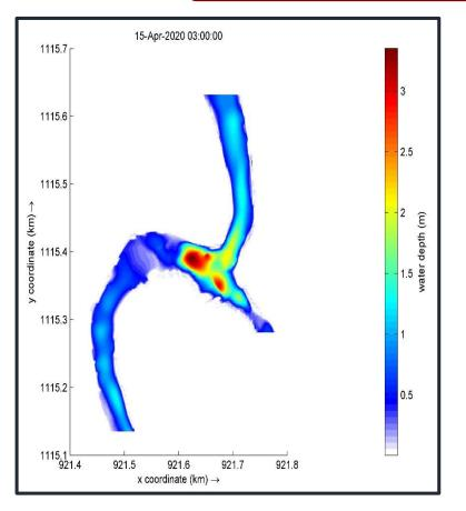
In the area of the rapids the water depth is 20 cm and in the area of the moya water depth depths are more than 3 m.
