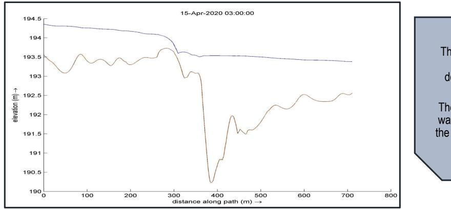
The graph shows the longitudinal profile from upstream to the downstream boundary, passing through the rapids.
