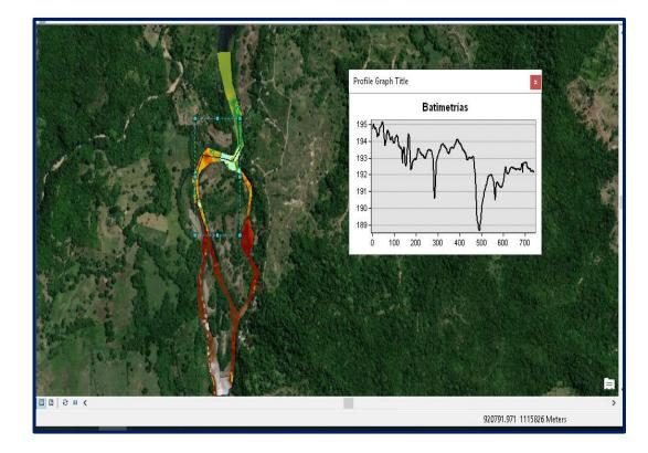
An IDW interpolation Python code was made where the elevation the bathymetries values were obtained from the RTK. The values were then subtracted from the depth of the echo sounder and finally interpolated using the Kriging in ArcMap.
