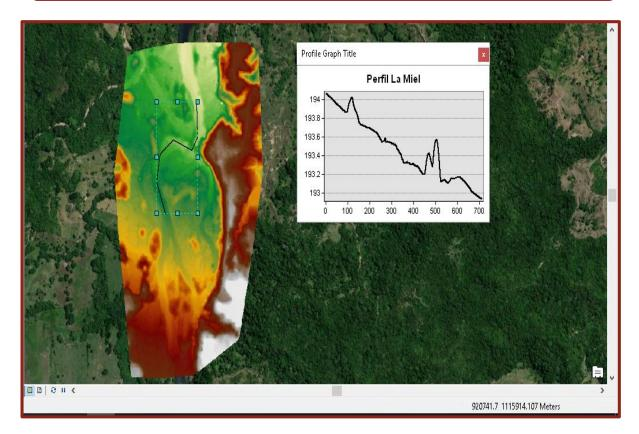
The images obtained from drones were used to generate the digital terrain image, which was processed using the Pix4D software.
