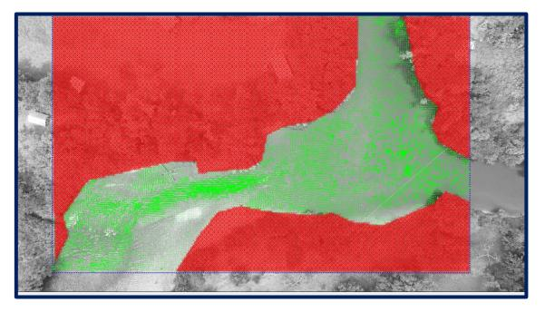
The velocity vectors were obtained processing the drones videos with the River 2.4.3 and PIVIab 2.00 Software using the Particle Image Velocimetry (PIV) technique.
