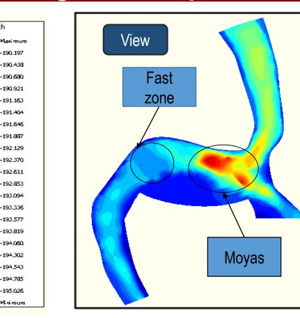
The figures show the plant view of the depth using a triangular interpolation of the topobatimetry of the "Moya de Jorge" section taking into account the mesh.
