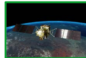
GoSAT satellite spectrometer lower precision, measures every 3 days
