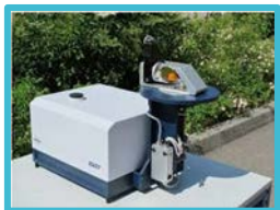
EM27/SUN portable ground spectrometer higher precision
