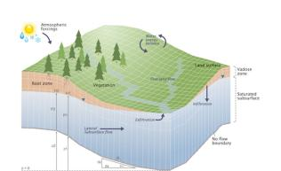
ParFlow: A fully integrated hydrologic model
