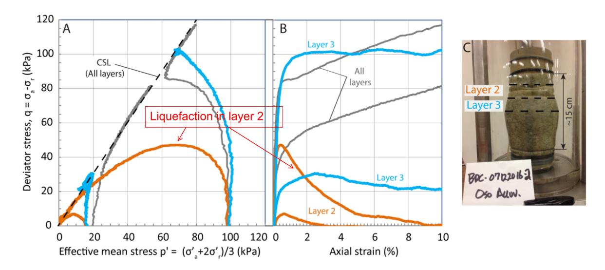
Triaxial tests show complete strength loss and liquefaction in select alluvial layers sampled from the slide site. Results from layer 2 (orange lines) and wrinkled membrane in photo indicate strength loss.
