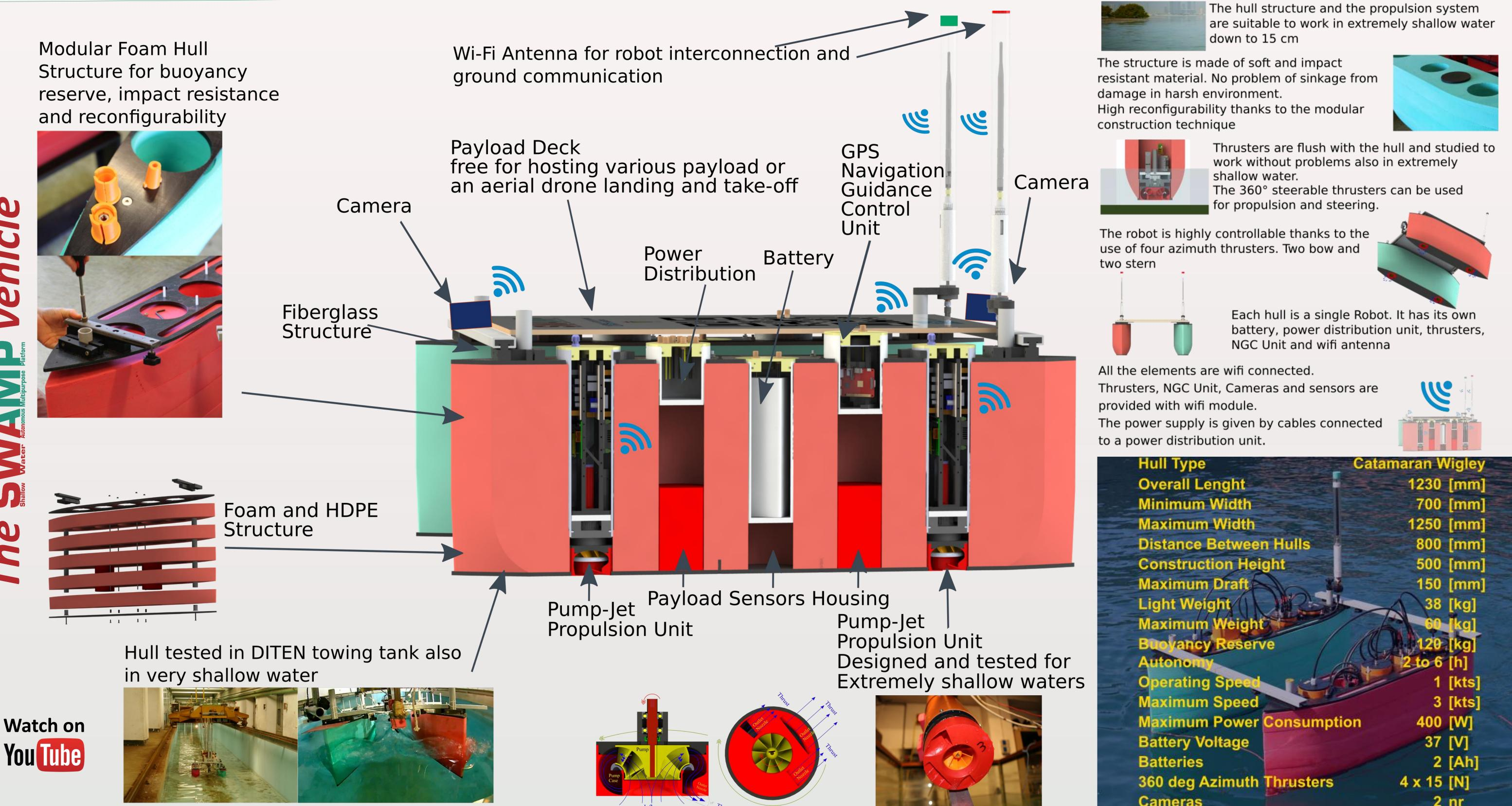
Hull foam is drilled to make SWAMP a completely modular catamaran able to host various types of tools: actuators, intelligent systems, samplers, and sensors that are, in this way, protected by the foam. This is studied to extend the ability of monitoring anthropogenic impact in hardly accessible harsh environments where commonly the vehicles do not access
