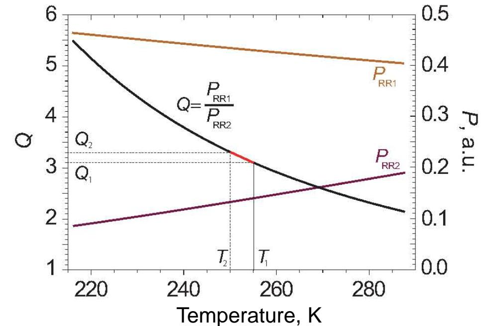
$$T(R) = -\frac{2a^2}{b \pm \sqrt{b^2 - 4a[c - \ln Q(R)]}}, \quad \sigma_T = \frac{\partial T}{\partial Q} Q \sqrt{\left(\frac{\sigma_{RR1}}{I_{RR1}}\right)^2 + \left(\frac{\sigma_{RR2}}{I_{RR2}}\right)^2} = \frac{\partial T}{\partial Q} Q \sqrt{\frac{1}{N_{RR1}} + \frac{1}{N_{RR2}}}$$
