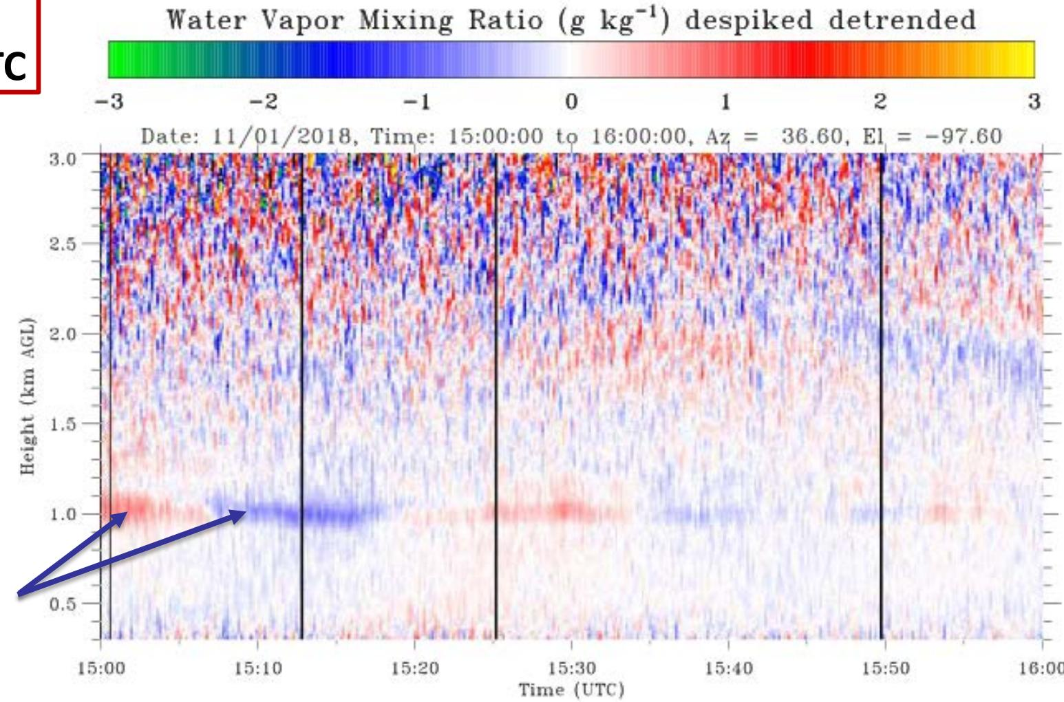
A gravity wave causes anti-correlated fluctuations in the temperature and WV mixing ratio
