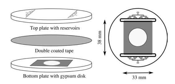
Microfluidic experiments designed to observe changes in size and shape as cylindrical disks (radius 10 mm) of gypsum dissolved for periods of up to 40 days.
