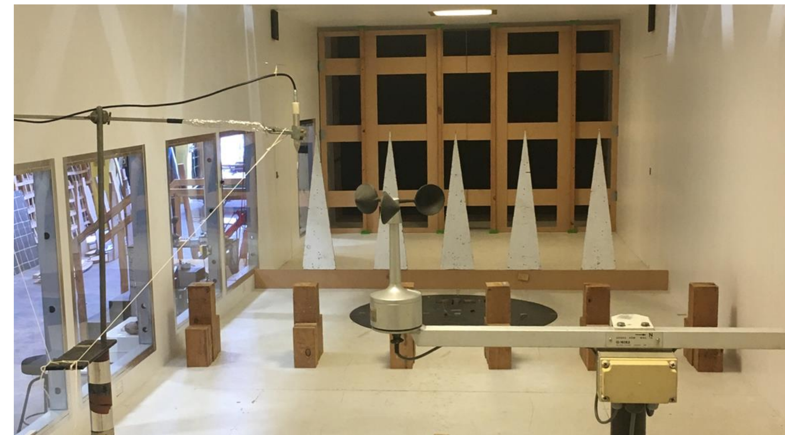
Figure 3. Example of wind tunnel setup for generating turbulence
