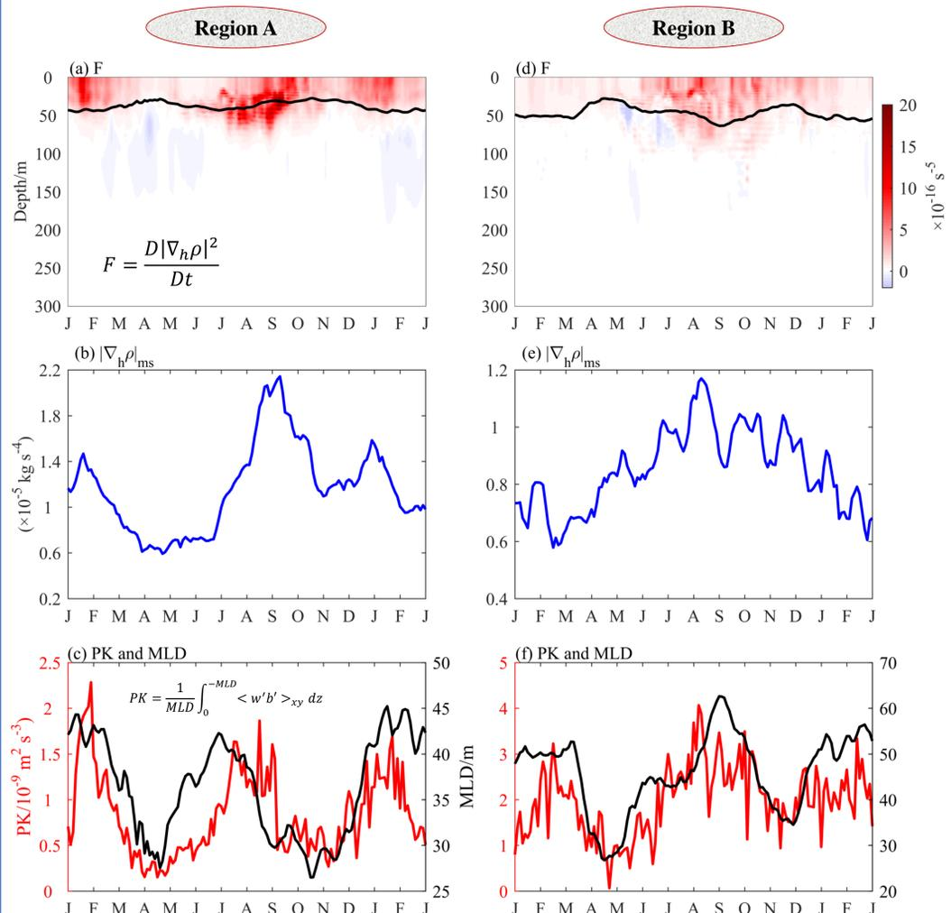
Figure.4. Time series of (a) region-mean of the frontogenesis  $F$  as a function of depth (the black denotes the region-averaged MLD), (b) region-mean horizontal density gradient integrated over MLD, (c) the rate of conversion of APE to EKE, PK (red) and MLD (black) in region A. (d)-(f) are the same as (a)-(c), but in region B.
