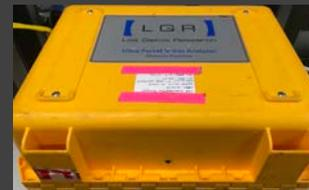
Fig. 2. Setup of the Los Gatos Research (LGR) ultra-portable greenhouse gas analyser for mobile measurements of CH<sub>4</sub> and CO<sub>2</sub> mole fractions. Measurements were georeferenced using a Hemisphere GPS linked to the instrument.
