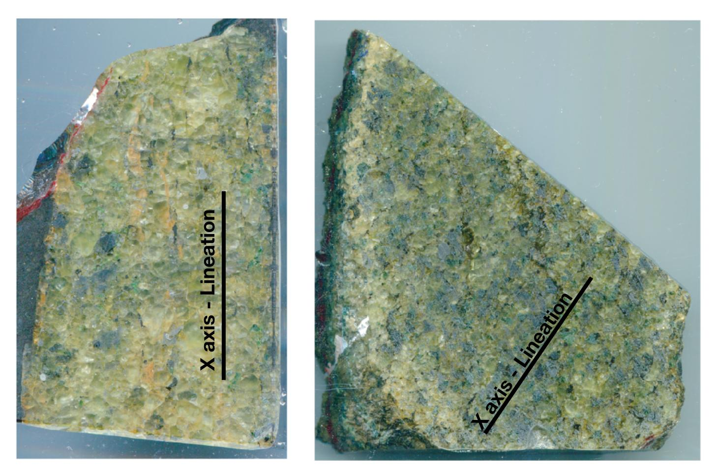
Examples of studied mantle xenoliths. The xenoliths are predominantly lherzolites. The slabs are cut parallel to the XZ plane (i.e. normal to the foliation and parallel to the lineation) of the spinel fabric ellipsoid. The elongation of spinel grains on the XZ plane define the X axis (black line) of the spinel fabric ellipsoid (mineral lineation).
