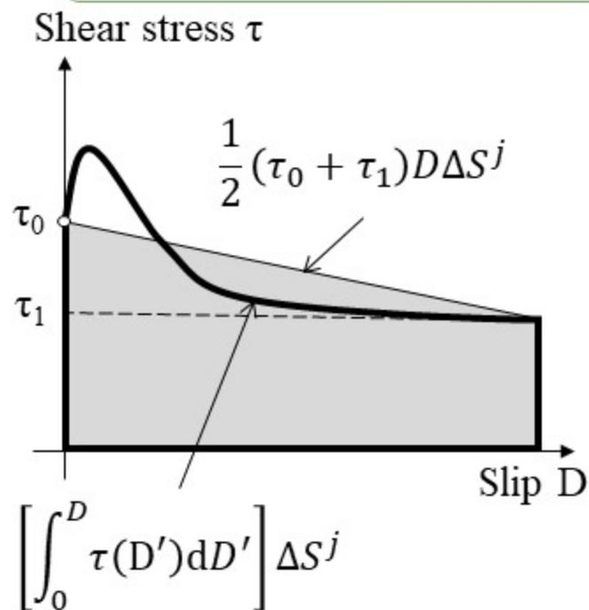
Strain energy released by an earthquake
