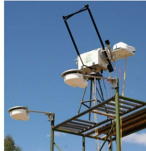
BSRN Station. (Baseline Solar Radiation Network). Measurement of Surface short wave and long wave solar radiation.
