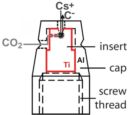
First, the sample can be injected as gas into the AMS, which upon interaction with sputtered  $\text{Cs}^+$  on a Ti target surface forms  $\text{C}^-$  (see reactions left).
