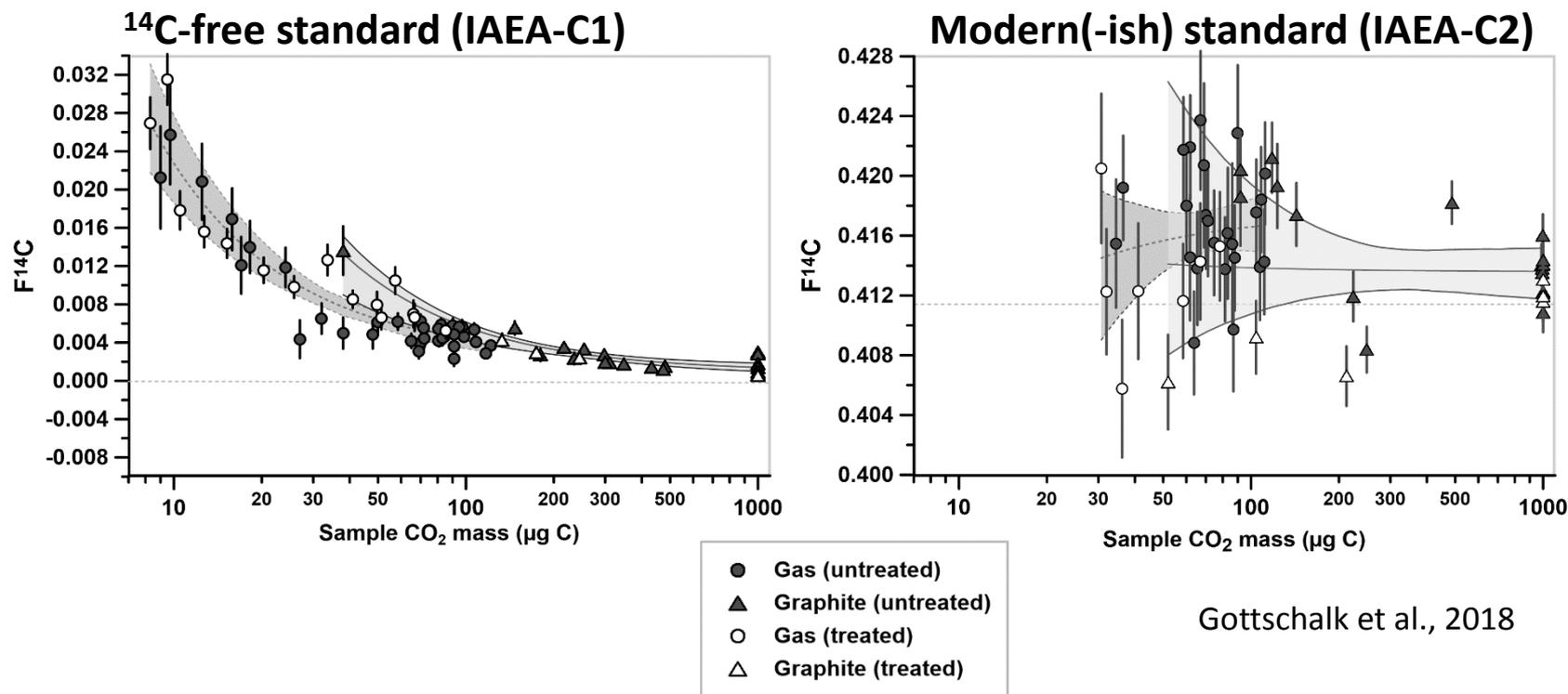
\*It is crucial to accurately determine the mass and F-modern of contamination of the MICADAS that has a strong effect on small and/or old samples
