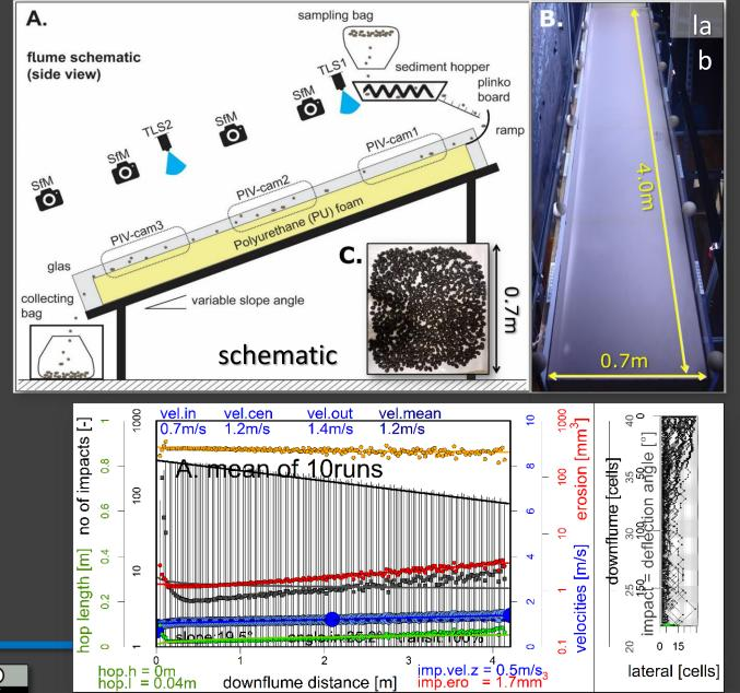
Erosion relations with slope and grainsize preliminary results
