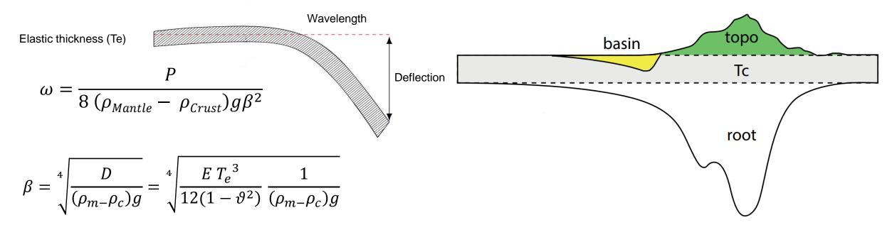
$(\rho_{Mantle} - \rho_{Crust})$  accounts for replacement of Mantle by a crustal rock or in other words deflected volume is filled by crustal rocks
