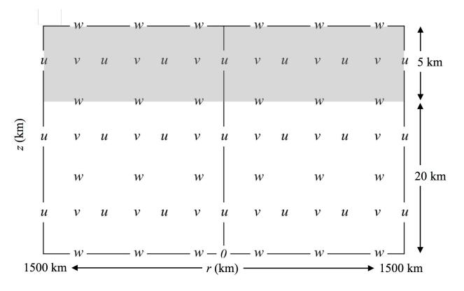
The model variables are placed on a staggered grid, whose alignment is shown in the figure above. Variables including  $\theta$ ,  $\pi$ ,  $q_v$  and  $q_l$  also sit on the grids of v.
