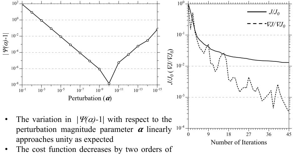
magnitude and the norm of the gradient by more than three orders in 45 iterations
