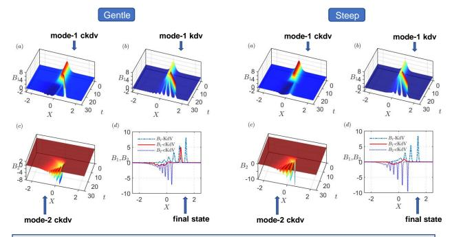
• A large-amplitude concave mode-2 wave is produced by an elevation incident mode-1 wave.
