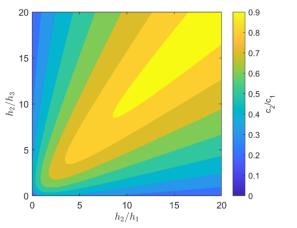
The ratio of mode-2 and mode-1 wave speeds  $(c_2/c_1)$  for a three-layer fluid model as a function of  $h_2/h_1$  and  $h_2/h_3$ .
