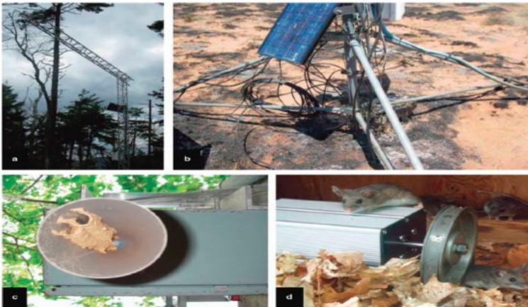
Figure 2. The measurements sensors can be damaged or destroyed by natural phenomena such as floods, fire, lightning strikes, and animal activity. [3]
