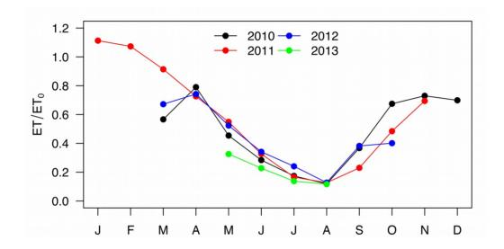
Seasonal evolution of the ratio of actual (ET) to reference  $(ET_0)$  evapotranspiration at the hillslope scale across 4 yr in Kamech. Actual evapotranspiration was measured by the flux tower installed on the northern hillslope of Kamech, whereas  $ET_0$  was measured by the meteorological station (adapted from Zitouna-Chebbi et al., 2018)
