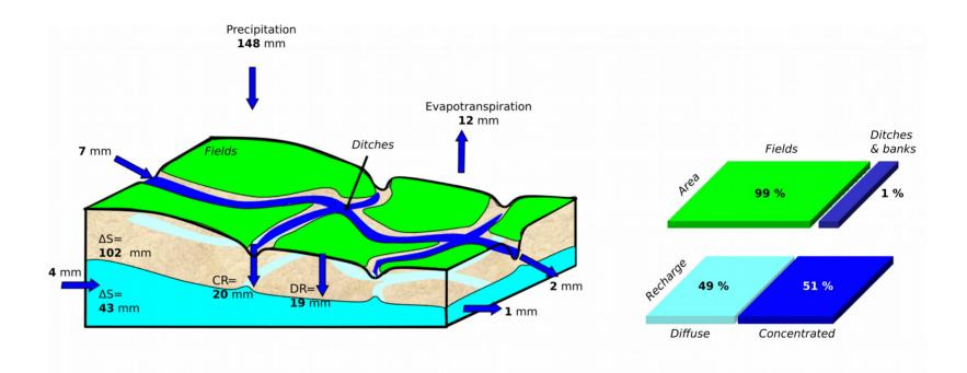
Water balance of the central depression of the Roujan catchment, calculated for the period of 7 to 20 Oct. 2005. CR, DR and  $\Delta$ S stand for concentrated recharge, diffuse recharge and water volume variations in groundwater and in vadose zone, respectively (adapted from Dagès et al., 2009).
