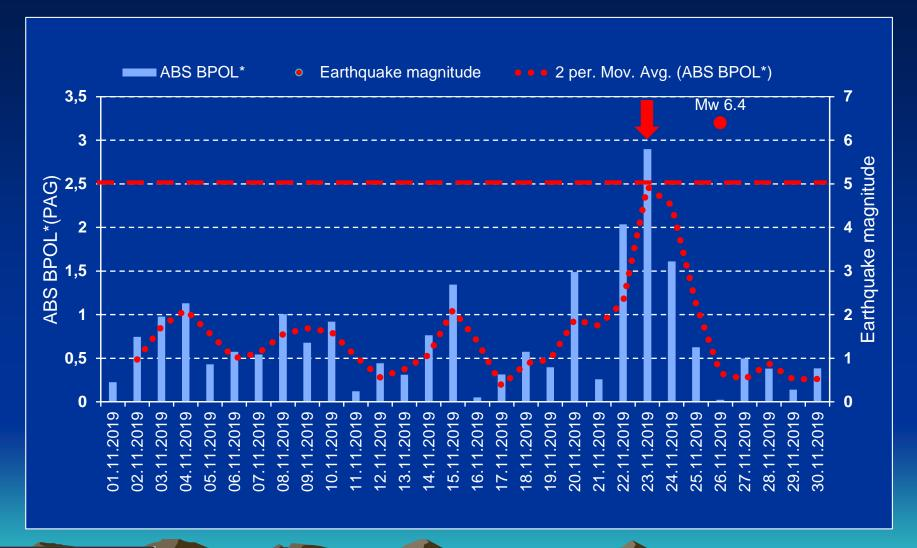
4. BPOL\*(PAG–SUA) time series obtained on the interval 01 – 30 November, 2019 Vertical red arrow emphasizes on 23 November, 2019 a pre-seismic anomalous signal, with 3 days before the onset of the Mw6.4 earthquake
