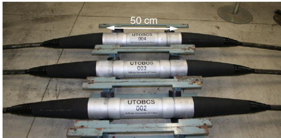
Fig. 5 A photograph of the cabled seismometers for deployment in the Japan Sea. The cabled seismometers have already connected to single armored optical fiber submarine cables. The size of the pressure vessels is 13 cm in diameter and 50 cm in length
