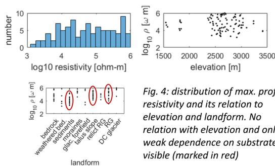
Fig. 4: distribution of max. profile resistivity and its relation to elevation and landform. No relation with elevation and only a weak dependence on substrate is visible (marked in red)
