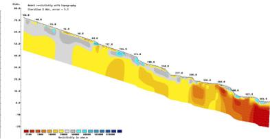
Fig. 7: eleven year repetition example from a very long transition profile from permafrost to non-permafrost conditions in Jotunheimen, Norway. This profile is regularly monitored (cf. Poster Hilbich et al., same session). Permafrost degradation is visible, but less evident from ERT, but was confirmed by borehole data.
