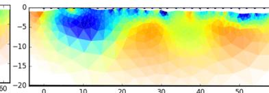
Fig. 8: ten year repetition example from Schilthorn (cf. Fig. 1). Here, the inversions were calculated with the BERT software (instead of Res2dinv, as for the other cases)
