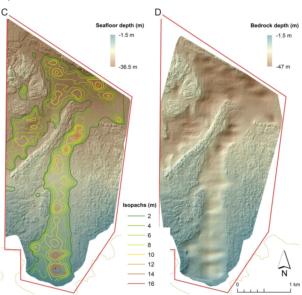
A. Thickness of sandy deposit below the northern margin of Gijón; B. Depth of the roof of these sediments in this area of the city; C. Bathymetry of the seafloor towards the N and thickness there of the unconsolidated sediments; D. Morphology estimated for the bedrock under the sedimentary filling.
