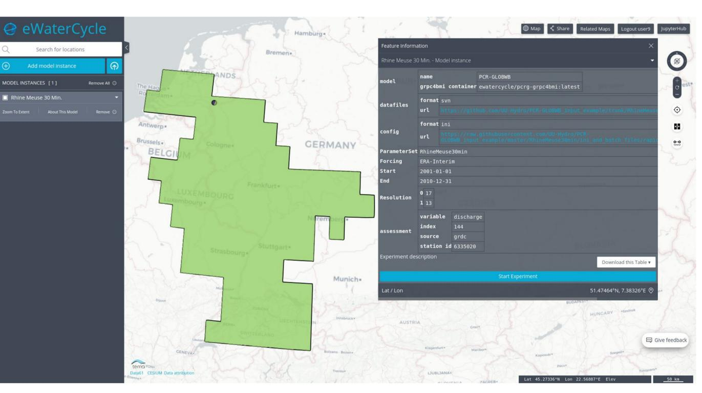
eWaterCycle is a framework in which hydrological modelers can, for example, compare and analyze the results of models that use different sources of meteorological data. The goal of eWaterCycle is to advance the state of FAIR (Findable, Accessible, Interoperable, and Reusable) and open science in hydrological modeling.
