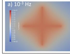
A time-harmonic vertical displacement is applied to the upper boundary of a sample containing two intersecting fractures, the resulting pressure is mapped at different frequencies.
