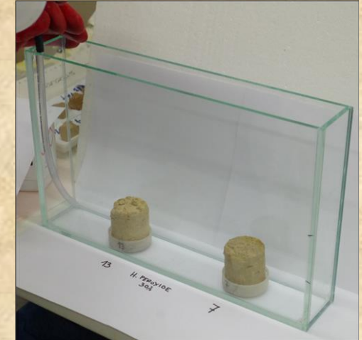
The setup for air slaking experiments
