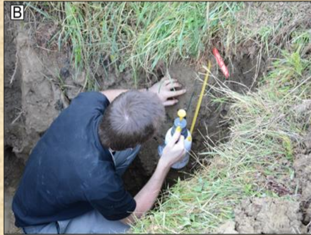
Field measurements of tensile strength (TS) and Relative Erodibility Indicator (REI)
