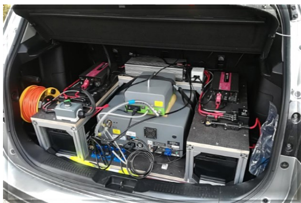
Figure 5. a. Mobile platform with b. Picarro G2201-i CRDS analyser
