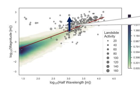
The vertical distance of each landslide to the trendline (its expected value) is a proxy for landslide activity.
