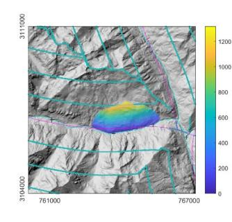
The difference between the medians of the two distance distributions serves as a proxy for the landslide displacement magnitude.
