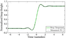
We use the above template to model all jumps from both, transponder phase  $\varphi_T$  and master phase  $\varphi_M$ . Afterwards, we can subtract the cleaned time series from each other. To do so, we need to interpolate the transponder measurements to the master time.
