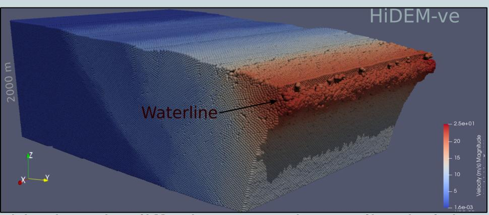
Thinning via cliff advance and waterline bulging occur in HiDEM-ve simulations. Shear band formation contributes to slumping & buoyant uplift, similar to observations at Helheim Glacier (Parizek et al., 2019).
