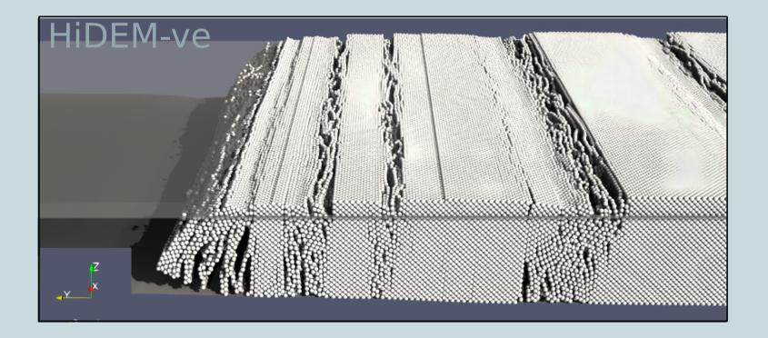
When sliding is induced, HiDEM-ve simulations show vertical crevassing and calving via block rotation.
