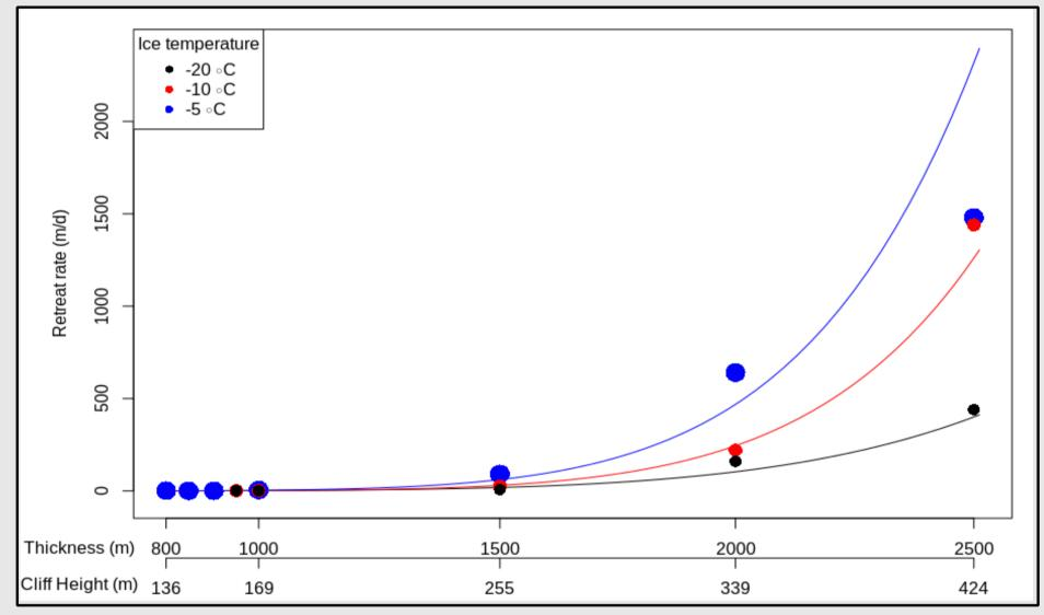
Retreat rates, derived with the consideration of viscious deformation and brittle failure, follow a power-law relationship with cliff height. Retreat rates quicken with warmer ice temperatures.
