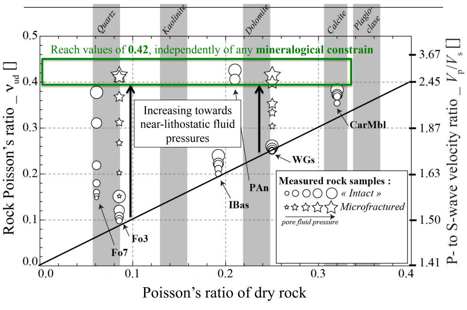
Measurements at varying fluid pressures in various isotropic crustal rocks ranging in mineralogy
