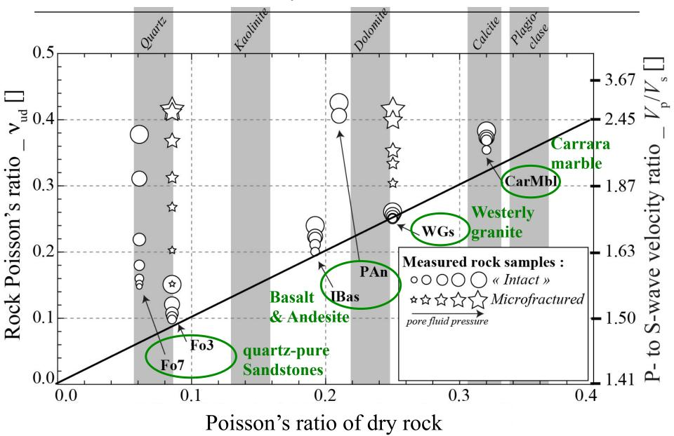
Measurements at varying fluid pressures in various isotropic crustal rocks ranging in mineralogy
