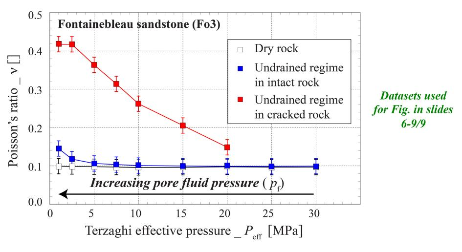
*Exemple* for a isotropic 100% quartz Fontainebleau sandstone, with large degree of cracking: Extreme Poisson's ratio in undrained regime at lowest effective pressure (i.e. near lithostatic pressure)
