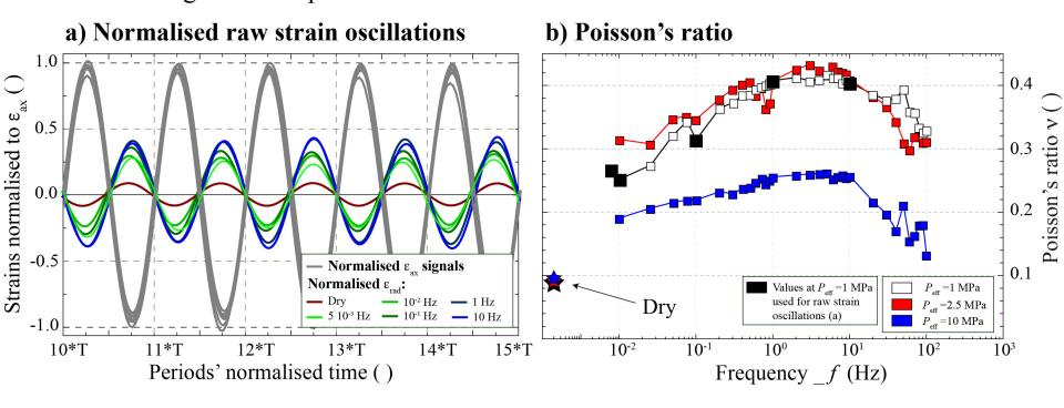
Exemplefor a isotropic 100% quartz Fontainebleau sandstone, with large degree of cracking:Poisson's ratio of up to 0.42 in undrained regime at lowest effectivepressure (i.e. near lithostatic pressure)Pimienta et al. (2018), GRL
