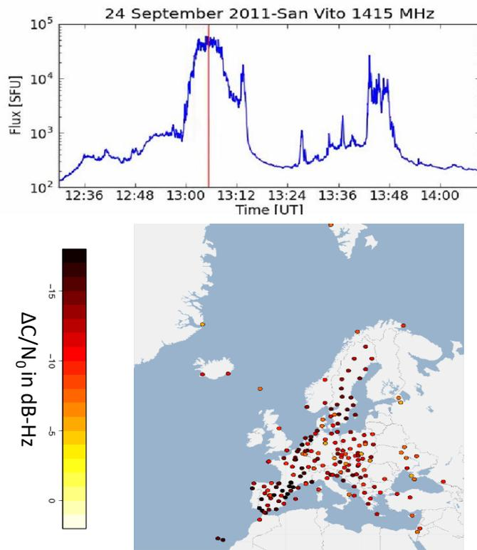
Figure 1: GPS signal reception fade at L2 for the EPN stations during the Solar Radio Burst of the 24<sup>th</sup> September 2011
