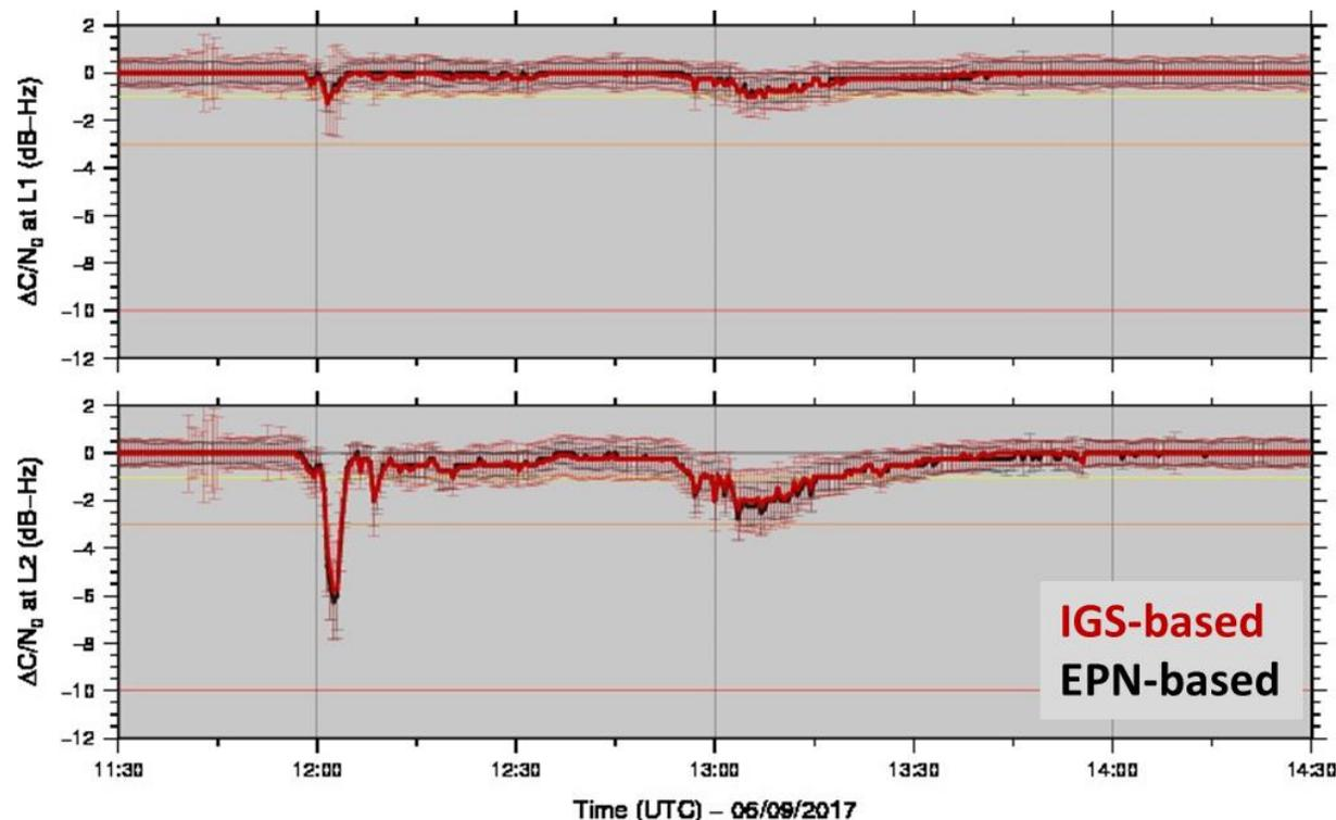
Figure 8: Carrier to noise density variations  $\langle \Delta C/N_0 \rangle_{L1,L2}$  over the IGS (in red) at daylight (sun elevation  $> 30^\circ$ ) and over the real-time EPN during the SRB of the 6<sup>th</sup> September 2017
