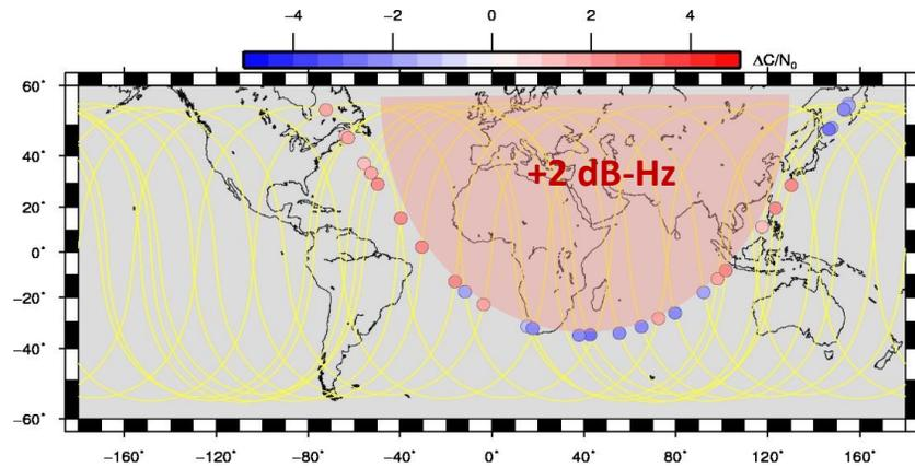
Figure 12:  $C/N_0$  variations of L1 C/A signals along the orbit of the Block IIF satellites using the IGS. It highlights the satellite locations of the flex power activation and deactivation on a typical day between the 27<sup>th</sup> Jan. 2017 and 14<sup>th</sup> of Feb. 2020
