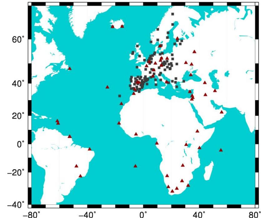
Figure 9: EPN (black) and IGS (red) stations used for the estimation of the European and Global  $\langle \Delta C/N_0 \rangle_{L1,L2}$  indexes during the SRB of the 6<sup>th</sup> September 2017
