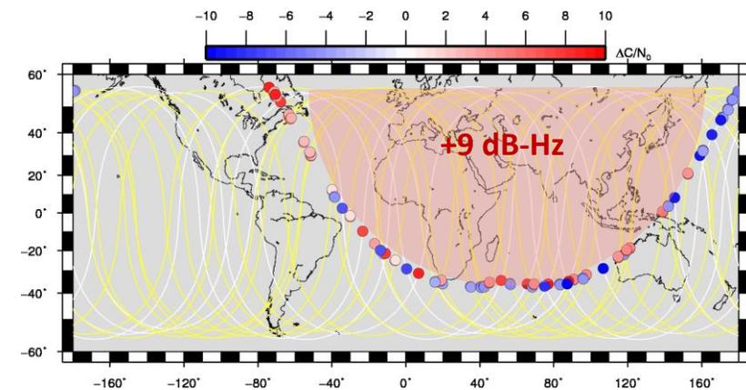
Figure 13:  $C/N_0$  variations of L2 P(Y) signals along the orbit of the Block IIF and IIR-M satellites using the IGS on a typical day since the 14<sup>th</sup> of Feb. 2020.
