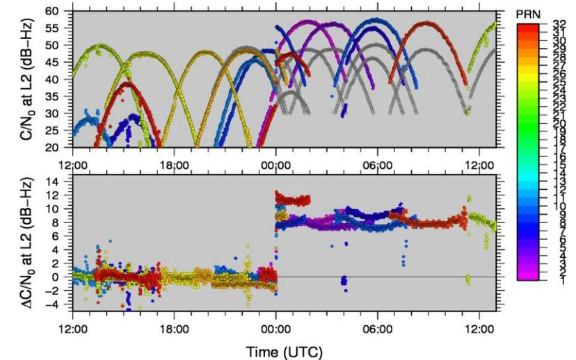
Figure 11: Flex power of the 14<sup>th</sup> Feb. 2020. Top plot:  $C/N_0$  observations from BRUX of the block IIF and IIR-M satellites (one colour per satellite) and their expected behaviour (in grey). Bottom plot: estimated  $\Delta C/N_0$  w.r.t. to the previous days
