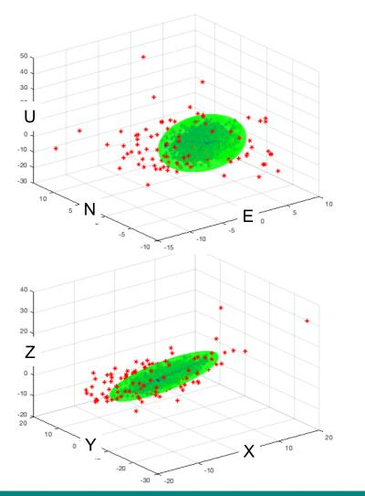
Note that since the ellipsoid is defined using the **full covariance matrix** of the residuals, it is also **oriented in the space** and **invariant in dimensions**.
