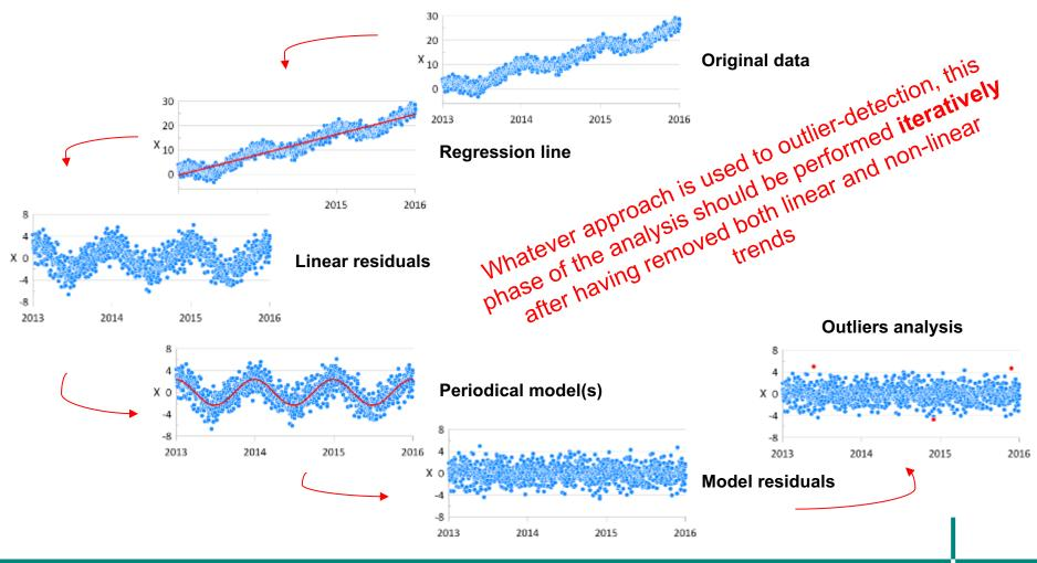
A new 3D approach to automated outliers rejection in GNSS time series. Tavasci L., luca.tavasci2@unibo.it
