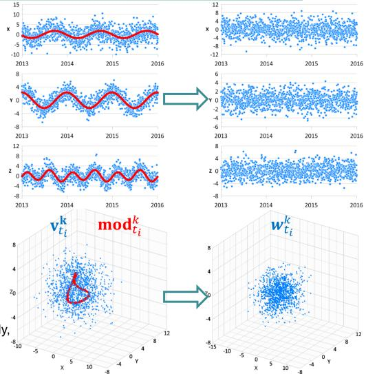
A new 3D approach to automated outliers rejection in GNSS time series. Tavasci L., luca.tavasci2@unibo.it
