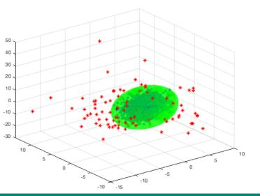
$\Sigma_{ww}^{k} = \frac{1}{n} \begin{bmatrix} \sum_{i} \left( w_{x_{t_{i}}}^{k} \right)^{2} & \sum_{i} w_{x_{t_{i}}}^{k} w_{y_{t_{i}}}^{k} & \sum_{i} w_{x_{t_{i}}}^{k} w_{z_{t_{i}}}^{k} \\ \sum_{i} w_{y_{t_{i}}}^{k} w_{x_{t_{i}}}^{k} & \sum_{i} \left( w_{y_{t_{i}}}^{k} \right)^{2} & \sum_{i} w_{y_{t_{i}}}^{k} w_{z_{t_{i}}}^{k} \\ \sum_{i} w_{z_{t_{i}}}^{k} w_{x_{t_{i}}}^{k} & \sum_{i} w_{z_{t_{i}}}^{k} w_{y_{t_{i}}}^{k} & \sum_{i} \left( w_{z_{t_{i}}}^{k} \right)^{2} \end{bmatrix}$
