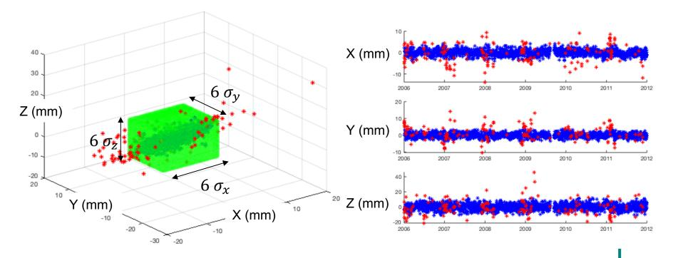
A new 3D approach to automated outliers rejection in GNSS time series. Tavasci L., luca.tavasci2@unibo.it
